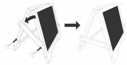
Begin by folding open the whiteboard and blackboard sides of the easel. Attach the two yellow arms, one on each side using four of the green bolts. Tighten all four bolts by rotating them clockwise.
